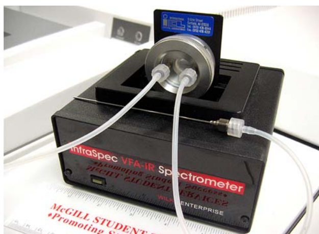
Fig. 1 The InfraSpec VFA-IR spectrometer with transmission flow cell and Luer-Lok needle used to aspirate the sample into the flow cell
